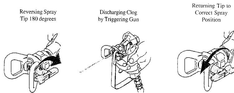
Figure 3-1—Unclogging RAC tip
